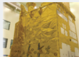
4 MLI Installation Configuration for GEO-KOMPSAT-2
