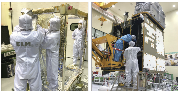
| MLI Installation Configuration of GODIK / GK2A Anti-static grounding
