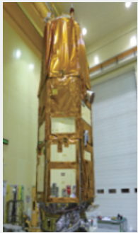
2 MLI Installation Configuration for KOMPSAT-3 / 3A
